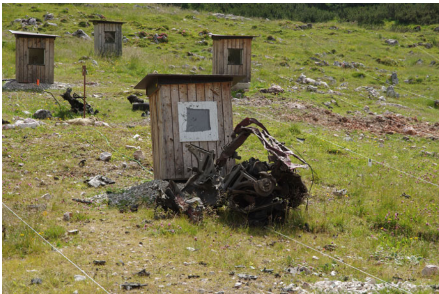
Fig. 7.3 Examples of car bomb fragments: parts of the front suspension and crash structure of the car stopped by a measurement box; just behind the box a wheel with the shock absorber; other fragments are distributed over the ground (Technical test center WTD 52 2013)
