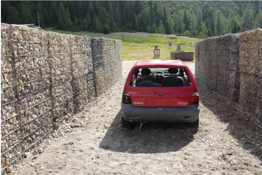
Fig. 7.8 Car loaded with 50 kg PETN behind the front seats in a simulated gateway of an asset. On the right and left hand sides there are gabions (hesco bastions) filled with stones with a diameter of 5 to 15 cm, height 2 m, width 1 m and length 10 m. The supermini car has a dry weight of 790 kg. All liquids and window glasses have been removed before the experiment (Technical test center WTD 52 2013 )
