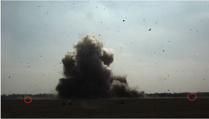
Fig. 6.3 Fragment launch distribution snapshot after a free field car bomb explosion, 1.1 s after the ignition. Besides the detonation products, dust of the sandy ground is visible over ground zero. The air is filled with thousands of larger and smaller fragments on all types of trajectories: from flat to very steep flight paths. Some characteristic fragments can be identified in videos, respectively on the picture. As an example, the two front shock absorbers with wheels attached are marked with red circles on their flat flight paths. In the corresponding video they first bounce to the ground, before, bouncing and rolling, they leave the visible area of the camera (Technical test center WTD 91 2013)
