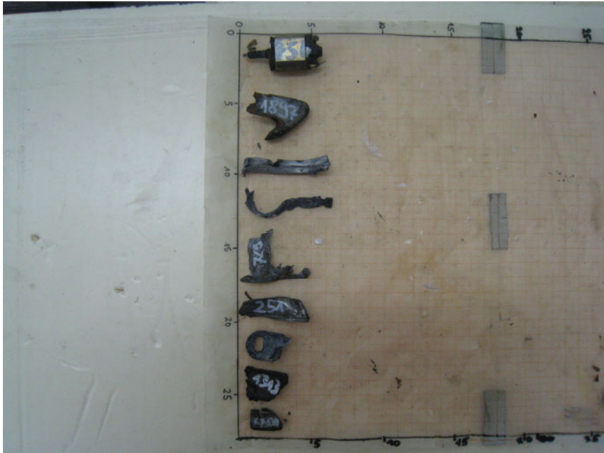
Fig. 7.2 Examples of smaller car fragments: at the top an electric motor (ca. 3 cm diameter) as used for the windscreen wiper or as window winder; beneath are other metallic fragments, some of them are bent by the explosion (Technical test center WTD 52 2013)
