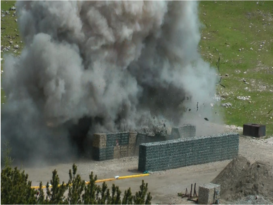
Fig. 7.10 Debris throw due to an explosion. This picture shows the same scenario as Fig. 7.8 during the explosion of the car bomb. The burst of the gabions and the resulting debris throw is clearly visible. The debris in this scenario consists mainly of rock pieces used to fill the structures besides the mesh wire that hold it. On the right hand side fragments of the car fly in driving direction. The cloud is mainly due to the crater dust (Technical test center WTD 52 2013)
