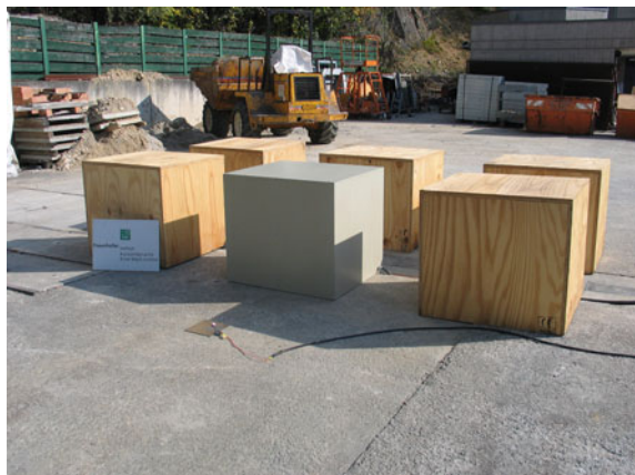
Fig. 8.5 Straight street with separated building blocks. The grey box is instrumented. The load is located in front of the building (Brombacher et al. 2009)
