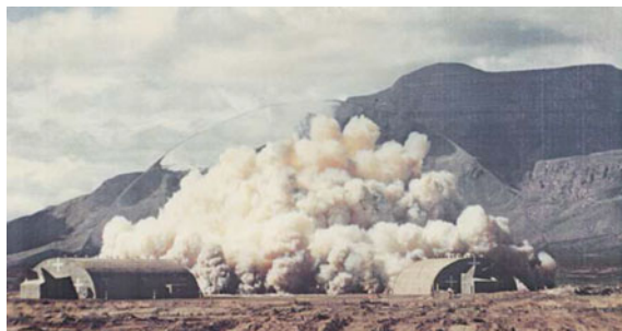
Fig. 6.7 Separation of blast wave from detonation products for ground burst. Picture likely to be taken during ESKIMO test series, see (Weals 1973) for ESKIMO I test series
