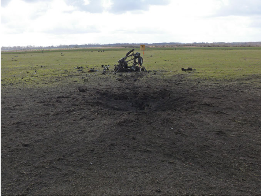
Fig. 7.11 Crater formation after car bomb free field explosion with 120 kg TNT. The ground consists of sand and topsoil and comprised only few stones. Behind the crater, fragments of the car are visible. The biggest fragment consists of the rear suspension, crash structure and a wheel. Smaller parts are widespread across the test site. In the middle of the background, a protective structure for the filming is visible (Technical test center WTD 91 2012 )
