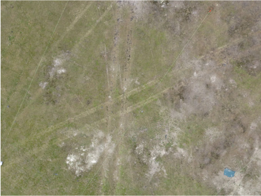
Fig. 7.7 Detection and localization of fragments after 2 test explosions. This picture shows a part of the test site that is 80 to 120 m apart from ground zero. The subdivision in 5^\circ angular sectors is clearly visible, as well as some medium and smaller fragments. The biggest fragment is the turquoise colored engine hood of one of the car bombs in der lower right part of the picture. This fragment was torn apart in one piece from the car. It is interesting that it is not much twisted like many other fragments. Such fragments are candidates for rather irregular distribution due to sailing effects. The composed aerial pictures allow to zoom in the pictures (Technical test center WTD 91 2014)
