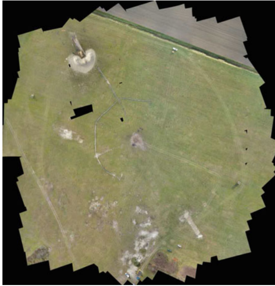
Fig. 6.1 Top view of an explosive test site after 3 explosive test events, taken with an aerial drone. Visible are the crater in the center, crater throw (ejections) and some of the large fragments of the car (direction 01:00 and 07:00). A close look reveals radial marking lines, which are used to locate fragments and debris within 5° sectors. The farthest thrown visible fragment is a turquoise colored engine hood (direction 07:30), ca. 100 m away from the explosion site. Source: Technical test center WTD 91 (Technical test center WTD 91 2014)
