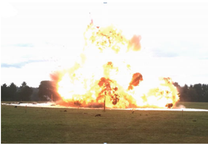
Fig. 6.2 Fireball, fragments and effects of blast expansion in case of car bomb explosion of 100 kg PETN ignited on the floor between front seat and rear bench. The sudden pressure rise generates the condensation disc on the ground. Diameter of fireball: ca. 10 m, time after ignition: 37 ms. Minor first fragments are visible in the left half of the picture (Technical test center WTD 91 2014)
