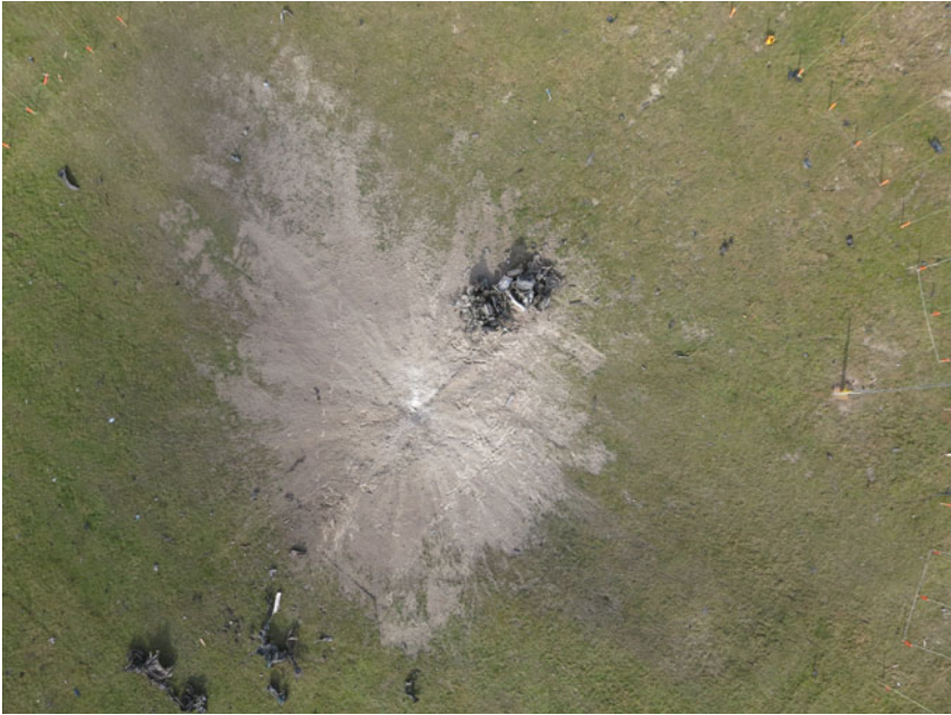
Fig. 7.12 Free field test site after two car bomb explosions with 100 kg PETN. It was taken with an aerial drone flying in a height of 30 m above ground zero. The crater and some big fragments are clearly visible. The big fragments consist mostly of the rear suspension, the crash structure and parts of the frame. Smaller parts are widespread across whole parts of the test site. The test site was subdivided in 72 angular sectors, each 5° wide. The orange poles and yellow ropes close to the crater are visible on the right side of the picture. This test arrangement improved the localization and classification of the fragments as well as the analysis of the aerial photos. The first 20 m around ground zero are excluded, because of the high explosive loading (Technical test center WTD 91 2014 )
